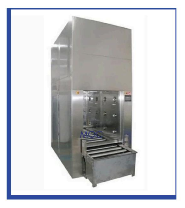
The De-Dusting Tunnel/Booth system is used to remove the loose foreign particles/dust present on the received material, which are brought into the warehouse area before they transferred into the quarantine area. Motorized roller conveyor transfers heavy load material from material loading area to dedusting chamber and then finally to the material unloading side.
